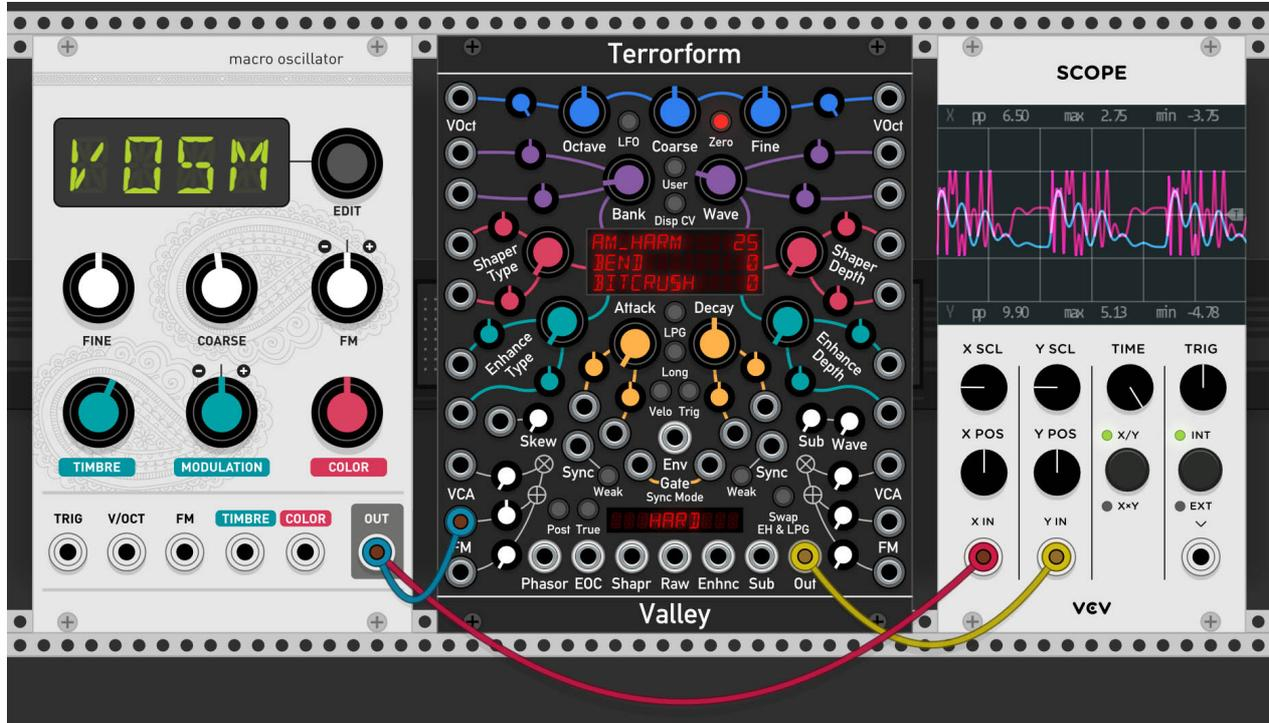
*Note:* The waveshaping result will depend on the peak-to-peak voltage and voltage offset of the input signal. For optimal waveshaping, the input signal should be  $\pm 5\text{v}$  peak-to-peak with no offset.
